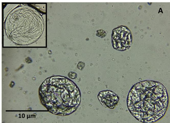
Fig. 1. Optical microscopy images: (A) PU microcapsules and (B) FTIR spectrum of PU showing typical polyurea bands.
